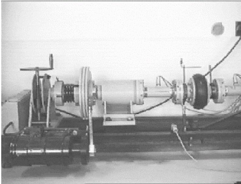
**Figure 3.** Picture of the stand “Elastic Coupling”
