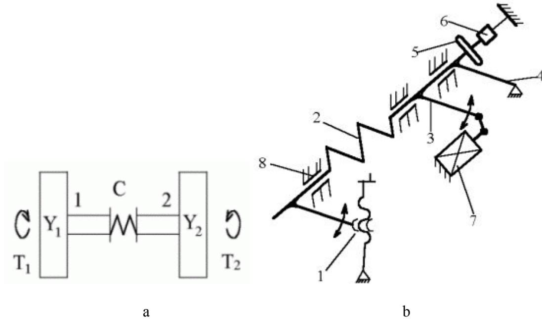
**Figure 2.** Representation of a dynamic model (a) and of a diagram of a stand for static and dynamic study (b); 1 – screw-and-nut gear, 2 – cylindrical spring, 3 – flat spring, 4 – strain measuring of the angle of torsion, 5 – elastic coupling, 6 – strain measuring shaft for measuring the torsion moment, 7 – electric engine with a crank mechanism, 8 – supports.
