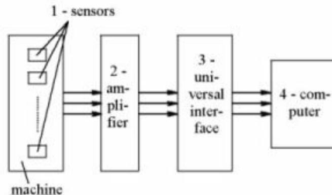
**Figure 1.** Diagram of measuring physical and mechanical parameters: 1 – sensor, 2 – amplifier, 3 – universal interface, 4 – computer.
