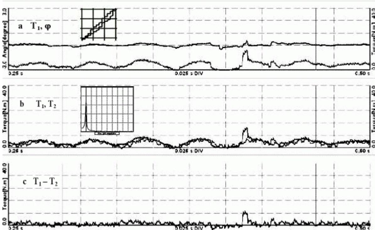
**Figure 4.** Results obtained with dynamic loading of a coupling; c and d – results of the dampening ability with static and dynamic loading.
